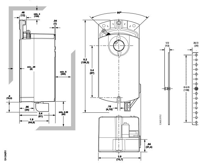
Figure 28. GDE131.1T, GDE131.1N, and Mounting Bracket Dimensions in Inches (Millimeters).
