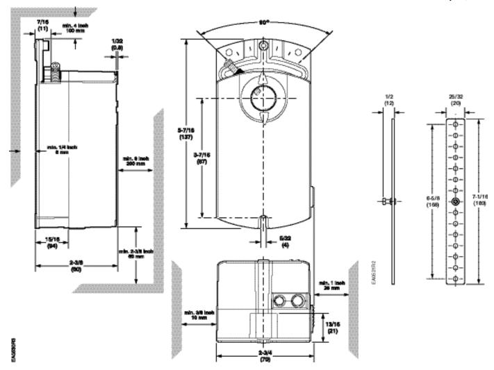
Figure 27. GDE/GLB Actuator and Mounting Bracket Dimensions in Inches (Millimeters).
