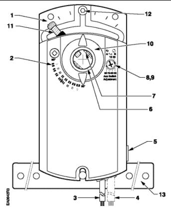
Figure 11. Parts of the Actuator.
