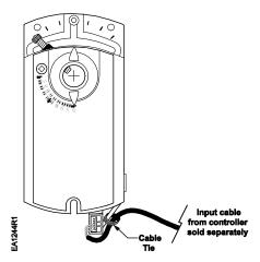
Figure 23. Input Cable Installed in Bottom Three Contacts.
