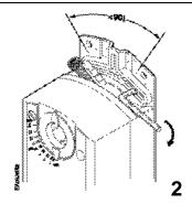
Figure 17. Moving the Mechanical Range Stop.
