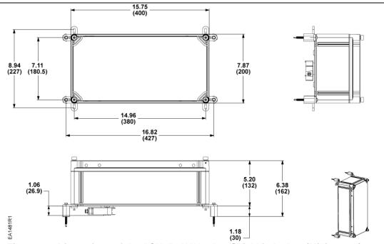
Figure 26. Dimensions of the ASK75.7U Weather Shield in Inches (Millimeters).
