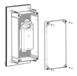
Figure 10. NEMA Type 4X Weather Shield.
