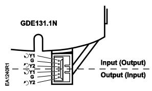
Figure 21. GDE131.1N Post Header AMP.
